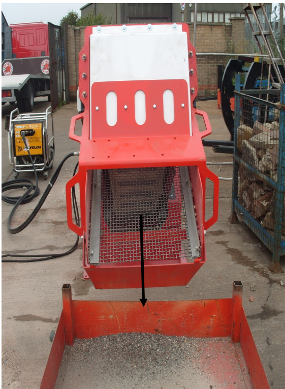
Oversized Material Direction
